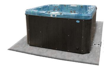
The foundation must extend 12" (1 foot/30.5cm) from the spa itself on all sides. this will distribute the spas weight across the whole foundation equally.
