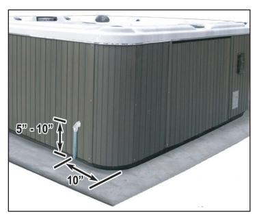
**Method 1:** Feeding the conduit through the cement slab to line up with your spas front right corner.
